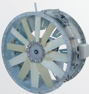
The Cimbria Axial Fan is a very efficient, low-pressure fan specially developed for aspiration from Cimbria continuous flow dryers. The Axial Fan is equipped with a robust nylon impeller, but, unlike all other Cimbria fans, the Varifan air volume regulator which is typically mounted externally is installed in the actual fan housing.
