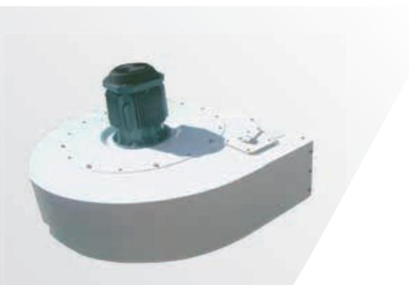
The Cimbria Centrifugal Fan type CM is a medium-pressure fan having backward curved impeller blades manufactured from steel plate. The impeller is self-cleaning and dynamically balanced. The CM Fan is typically used as an aspiration fan on a Cimbria cleaner or as an aeration fan in e.g. silos or flat storage. As standard it is equipped with throttle valves, but it can also be supplied with the specially developed Varifan.
