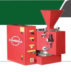
The CC Lab is a manually operated Centricoater to be used in a laboratory or breeding station for coating of single batches.
