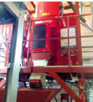
Saaten Union, Romania - Batch Treater CC150 Saaten Union, Romania - All Elevators were replaced with modern and gentle conveying Pendulum Bucket Elevators
