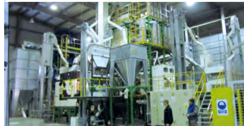
Saaten Union, Romania - Batch Treater CC150 Saaten Union, Romania - All Elevators were replaced with modern and gentle conveying Pendulum Bucket Elevators
