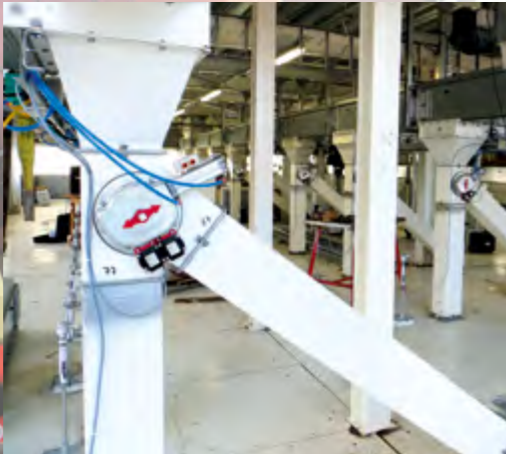
Distribution conveyors on the ceiling of the silo
