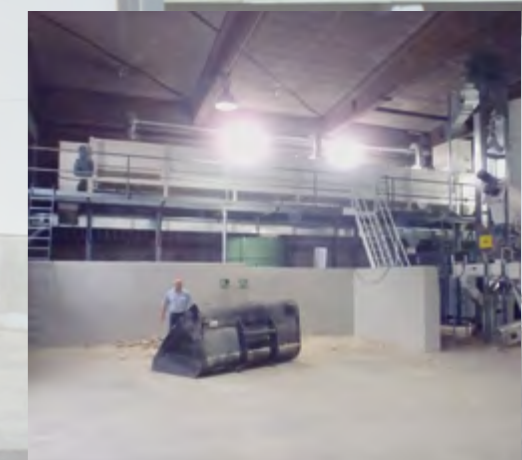
This picture shows most of the plant, with the belt dryer in the background and the large reception silo on the far right.
