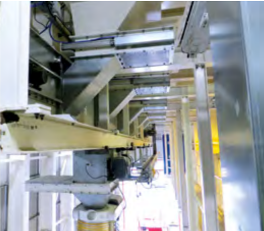
Loading facility featuring mobile conveyor with Moduflex loading chute
