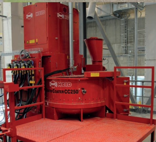
Chemical treatment 18 t/h
