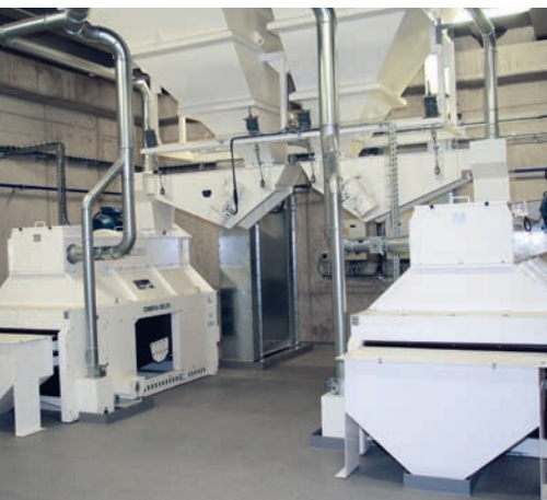
Shelling and pre-cleaning, 40 t/h
