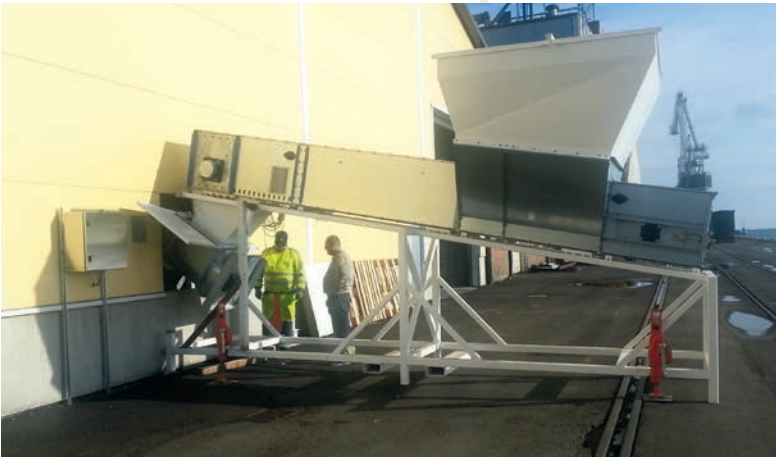
Chain conveyor 300 TPH from the ship hopper to the storage facility
