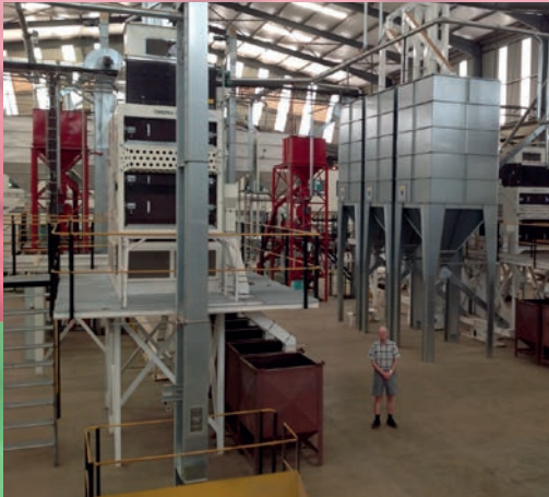
The new seed plant in Malawi consists of 2 processing lines, each for processing 10 t/h wheat. One line is additionally equipped for maize seed processing of 4 t/h in 3 grades.
