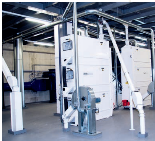
Calibration, 8 t/h in 3 grades
