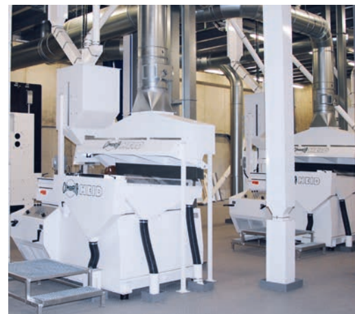
Fine cleaning and gravity separation 8 t/h
