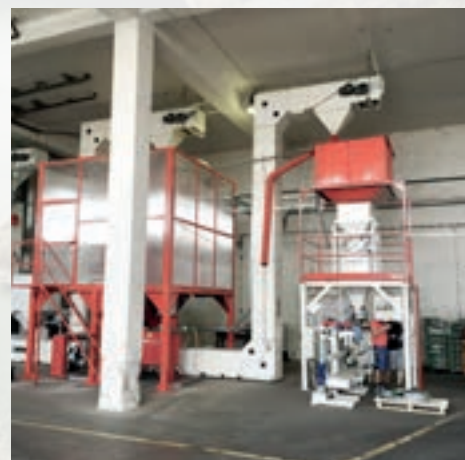
Pendulum bucket elevator for gentle conveying
