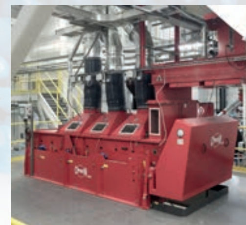
Cimbria jog conveyor dryer and belt feeder with burner control system and automated control system for gentle drying
