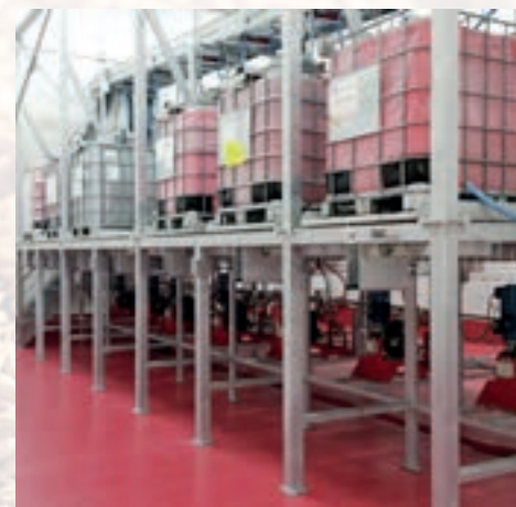
Pumping system with 7 dosing lines, each with 2 IBC tanks
