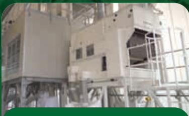
**CIMBRIA DELTA CLEANER** swiftly sorts material by size and eliminates flakes outside the tolerance range. An intake and exit system then purifies the material of dust and other light contaminants.
