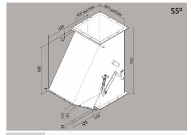
LN1052 Manually LN1054 Manually with indication LN1058 Pneumatically
