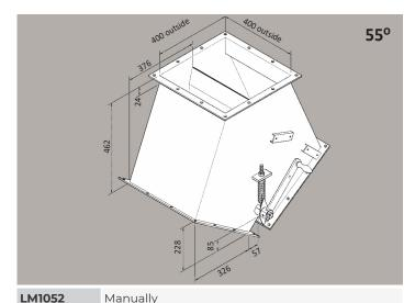
Manually LM1054 Manually with indication LM1058 Pneumatically
