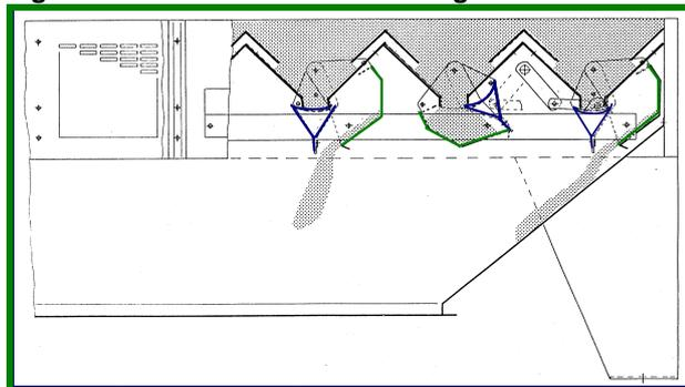
The size of the discharge apertures and -containers is the same for all models of dryers only the number varies as indicated in table 1.
