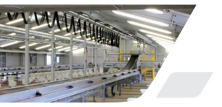
Corn is delivered to the silo cells by means of a belt conveyor. Belt conveyors are equipped with manually or electronically positioned discharge cars. The bins are filled through inlet pipes which are designed and connected to the filling chutes of the cells for very gentle product handling. The silo hoppers are designed to be completely self emptying. The outlets can be equipped with pneumatic or motor controlled shutters for capacity control.
