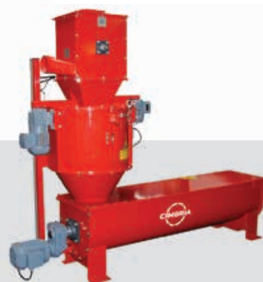
CONTINUOUS CHEMICAL TREATER For chemical treatment to protect kernels.
