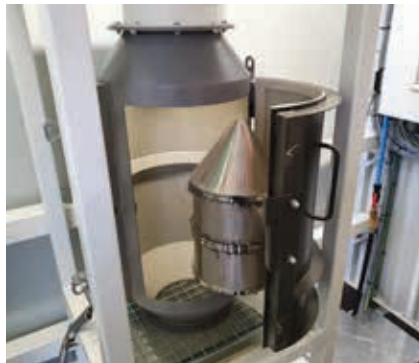
PIPE MAGNET To remove metallic parts.
