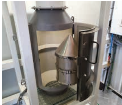
PIPE MAGNET To remove metallic parts.
