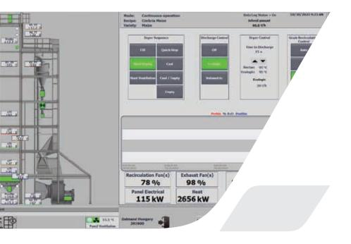
Dryers require precise monitoring and control for optimal performance. Sensors track temperature, humidity, and airflow, enabling automated controls to adjust heat and cycles. This ensures efficient drying, energy conservation, and product care, while preventing overheating and potential fire risks.
