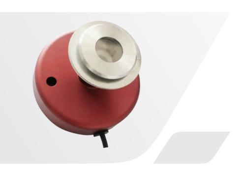
The CIM Safe infrared spark detection system secures at risk fire areas. A compact die cast sensor housing protects the infrared sensor from scratches. It connects to a control unit monitoring for sparks or fire, triggering alarms and shutting down equipment to prevent damage.
