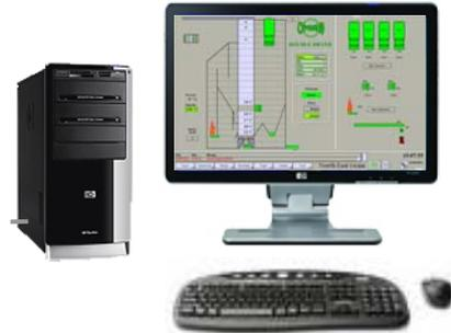
Start-up of the dryer is done in only 3 steps. First start Fans then Burner and when temperature is right then start the Discharge.
