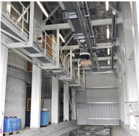
Modulflex loading chutes for dust-free outloading of pellets at Mysen Moelle
