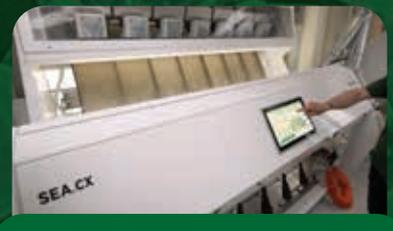
**CIMBRIA SEA.CX** optical sorter utilises the most advanced technology on the market, featuring high-definition Full-Color cameras to separate PET flakes into two homogenous colour fractions: clear and light blue. Our strategic balance of these fractions meets the colour standards of the blends used for sheet production.
