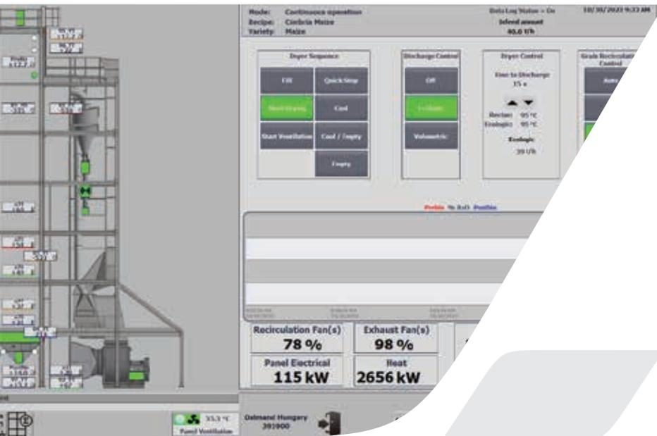
Dryers require precise monitoring and control for optimal performance. Sensors track temperature, humidity, and airflow, enabling automated controls to adjust heat and cycles. This ensures efficient drying, energy conservation, and product care, while preventing overheating and potential fire risks.
